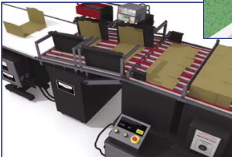
Its combined characteristics of high friction and abrasion resistance make the Linatex® backing ideal for box folding applications.
